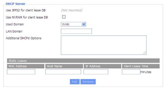
Use NVRAM for client lease DB: users can store data to the system NVRAM area is enabled Used domain: users can select here which domain the DHCP clients should get as their local domain. This can be the WAN domain set on the Setup screen or the LAN domain which can be set here.
