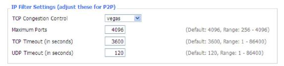
**IP Filter Settings (adjust these for P2P):** If you have any peer-to-peer (P2P) applications running on your network please increase the maximum ports and lower the TCP/UDP timeouts. This is necessary to maintain router stability because peer-to-peer applications open many connections and don't close them properly. Consider using these:
